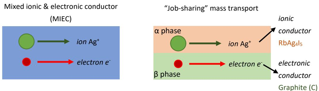
**Figure 1** Chemical diffusion in MIEC and job-sharing composites.
